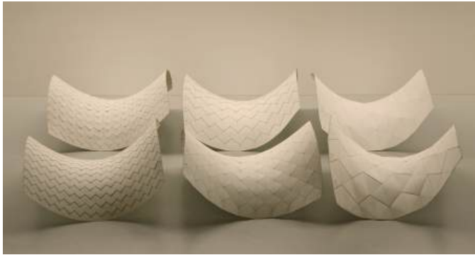
Figure 12: Hyperbolic paraboloid models of different tessellation density made by the traditional “Gluing Tab” method (front row) and the proposed “Double Shell” method (back row).
